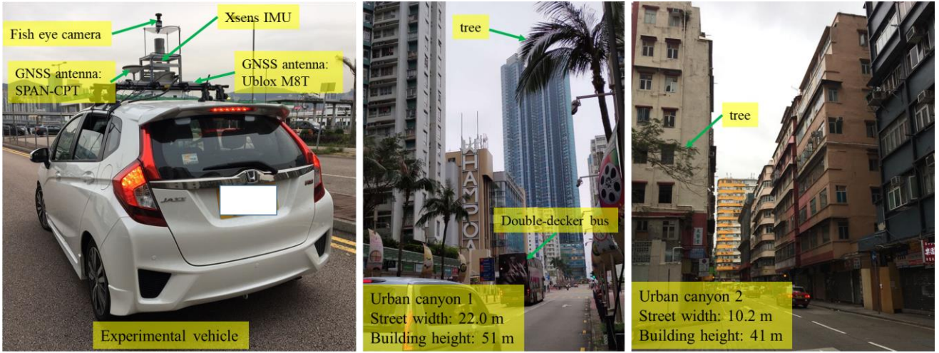
Fig. 6. Experimental vehicle and sensor setup in left-hand side figure. Tested scenarios of urban canyon 1 and 2.
